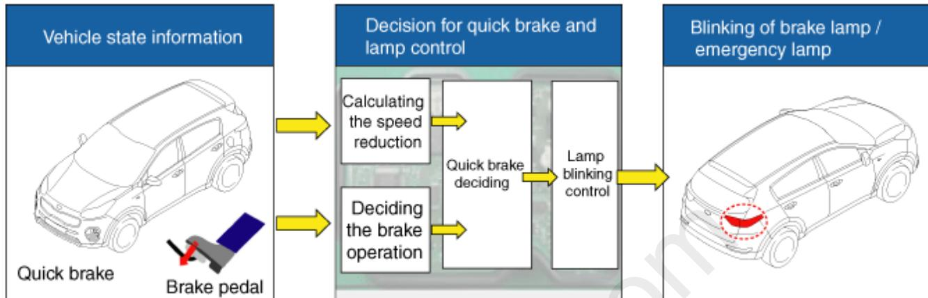
1. Basic function (Blinking the brake lamp/emergency lamp)
